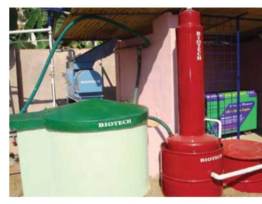
operation fuel in generators. Before feeding biogas as the fuel in generator, the gas has to be passed through a gas scrubber to remove unwanted particles, gases, moisture, and so on.
